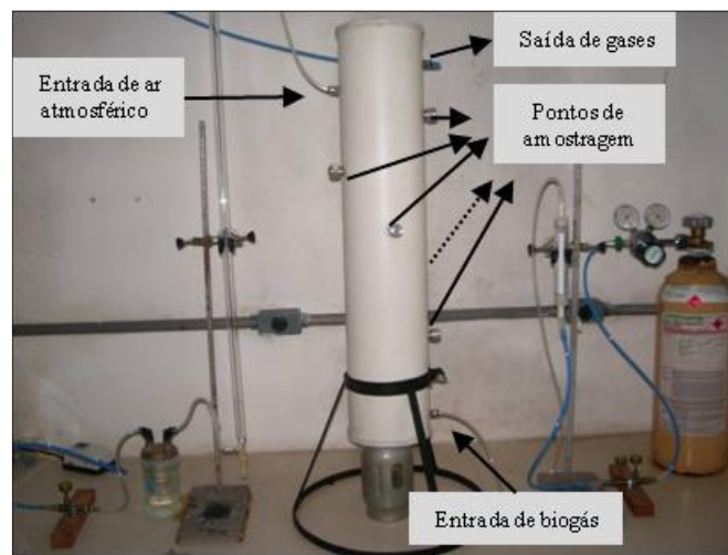
Figura 6. Coluna experimental de Salim (2011)
